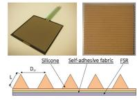
The silicone ridges affect the magnitude of grip and slipping frequency of an object. The skin with Drr = 4mm performs better in differentiating both weights and slippage frequencies.
